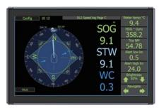
The SKIPPER DL2 is a Dual Axis Doppler Speed Log, working on the doppler principle, providing longitudinal and transversal ship's speed (STW and SOG) and distance relative to sea water. In addition the DL2 have the docking functionality providing the third axis. The SKIPPER DL2 gives accurate navigation parameters, measured as they happen, and presented in a logical, user-friendly way.
